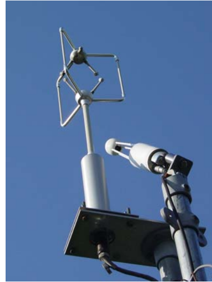
Eddy covariance system consisting of an ultrasonic anemometer and infrared gas analyzer.
