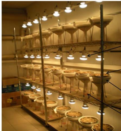
Light bulbs Sample container with soil sample Plastic funnel Collecting vessel with preservative
