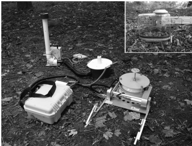
Open dynamic chamber systems from different manufacturers. PP-Systems CFX-1 at the back and ADC SRS-1000 in the small figure. Automatic closed dynamic system Li-Cor Li-8100 chamber at the front is based on closed dynamic technique.
